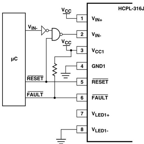
Figure 73c. Safe hardware reset for inverting input configuration.
