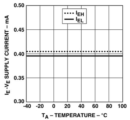
Figure 14. I<sub>E</sub> vs. temperature.
