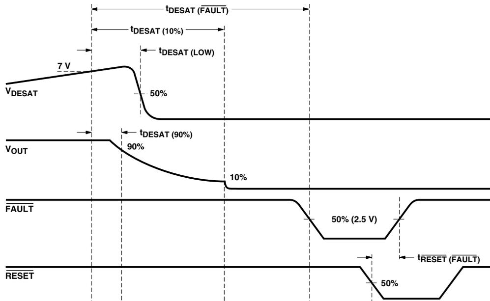
Figure 56. Desat,  $V_{OUT}$ , fault, reset delay waveforms.
