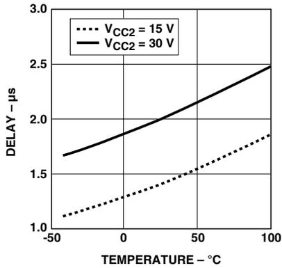
Figure 24. DESAT sense to 10%  $V_{out}$  delay vs. temperature.
