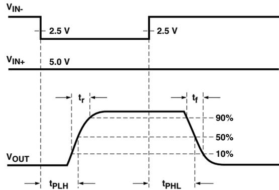
Figure 55.  $V_{OUT}$  propagation delay waveforms, inverting configuration.
