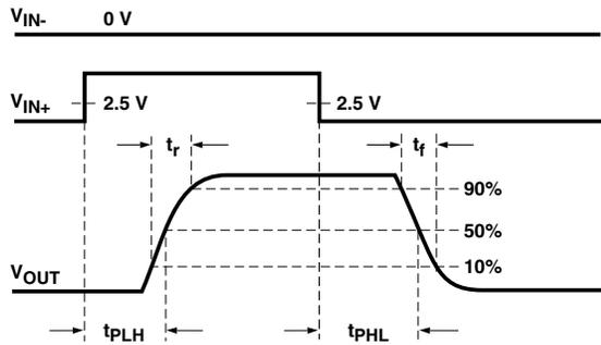
Figure 54.  $V_{OUT}$  propagation delay waveforms, noninverting configuration.
