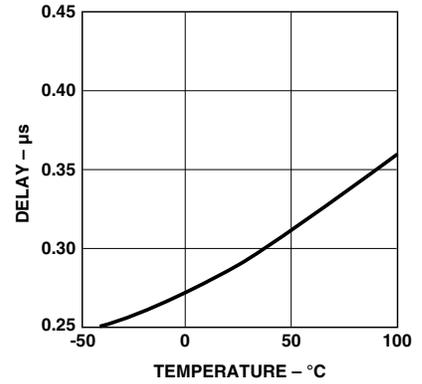
Figure 23. DESAT sense to 90%  $V_{out}$  delay vs. temperature.
