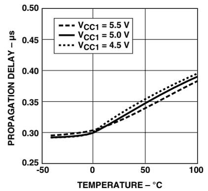
Figure 20. V<sub>IN</sub> to low propagation delay vs. temperature.
