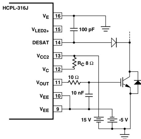
Figure 74. Use of  $R_C$  to further limit  $I_{ON,PEAK}$ .
