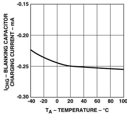
Figure 13. I<sub>CHG</sub> vs. temperature.
