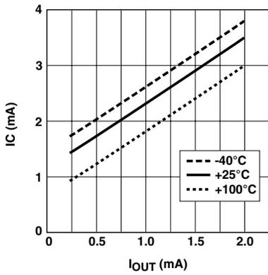
Figure 15. I<sub>C</sub> vs. I<sub>OUT</sub>.
