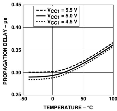
Figure 19. V<sub>IN</sub> to high propagation delay vs. temperature.
