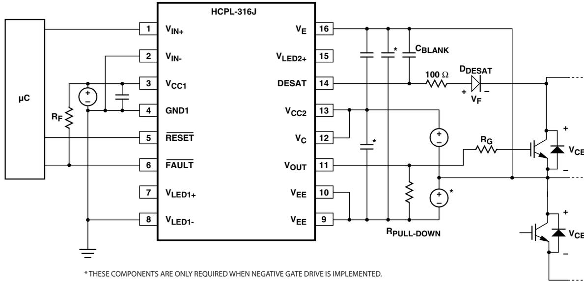
Figure 1. Typical desaturation protected gate drive circuit, noninverting.
